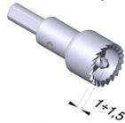
*This operation will not damage the thread on condition that the guide helix point is set in such a way that it does not protrude by more than 1÷1,5 mm (3/64"÷1/16") over the saw teeth.*
