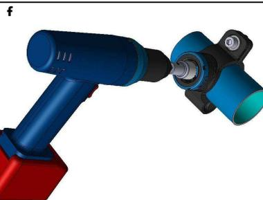
**4.8 Eliminate the burr after holing and carefully clean out all residues due to this operation (g).**
